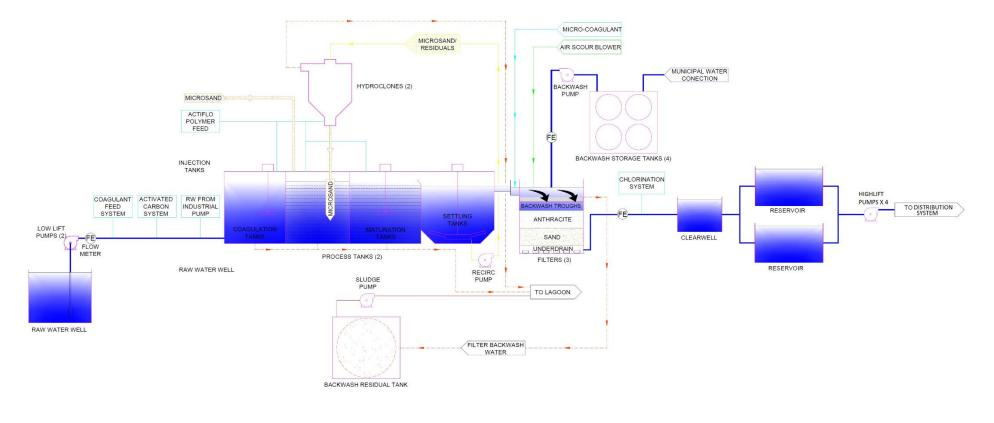
SIMPLIFIED PROCESS FLOW DIAGRAM NANTICOKE WATER TREATMENT PLANT
