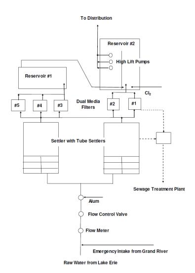
Figure 1: Dunnville Water Treatment Plant Schematic
