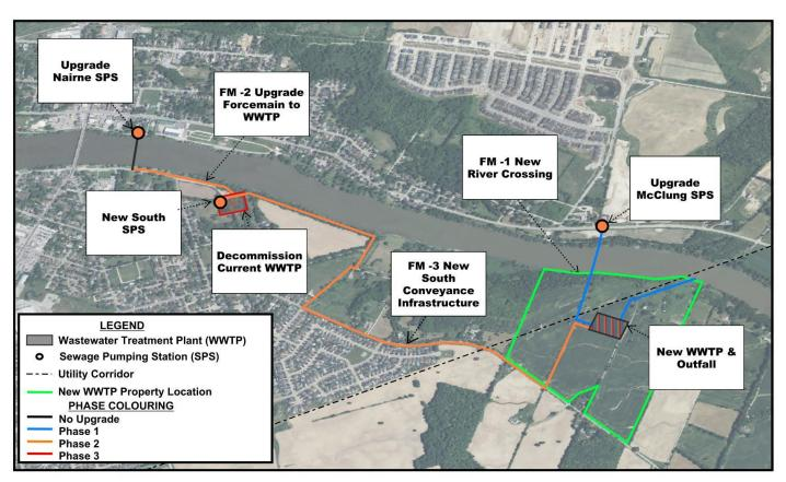
\*Note that the exact location of the New Wastewater Treatment Plant on the property, as well as the location of the outfall are conceptual in nature. The exact location will be confirmed during detailed design.
