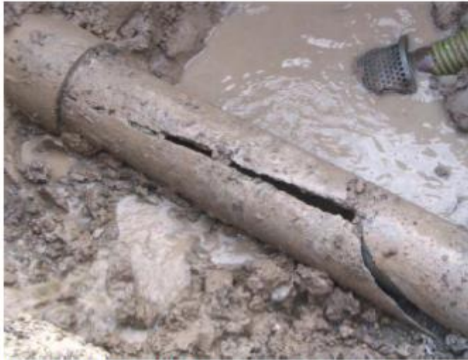
Figure 3: Longitudinal watermain break with evident Contamination.
